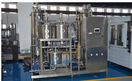
Figure 4. Mixing and carbonation equipment for a carbonated route; omit this stage for a still recipe where not required.
